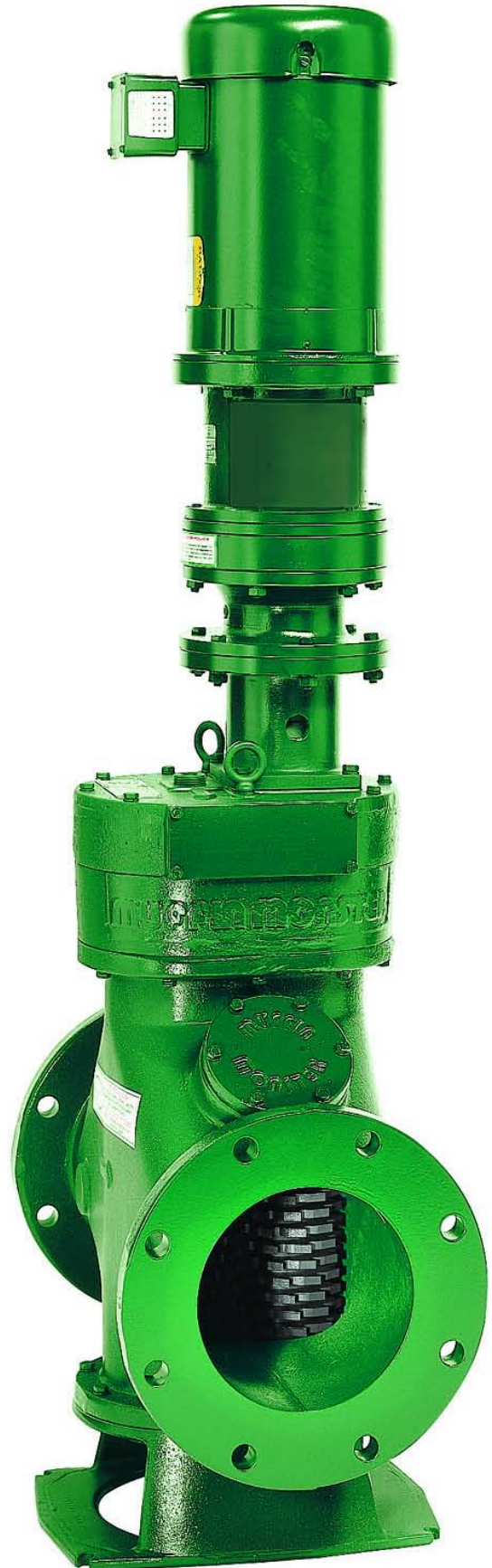
Dual-shafted Muffin Monster Model 30004 installed here has design flow rate of 800 gpm, and pressure drop of 1.60 psi. Model is available in flow rates ranging from 400-1200 gpm.
