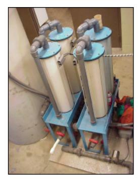
Influent to the EC System moves through stages of electrocoagulation, separation, and evaporation. pH is adjusted in a holding tank before it is pumped to the EC cells.
