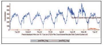
Concentrations of H<sub>2</sub>S entering the system typically range from 300-800 ppm. In recent actual odor log data for one of the towers, covering a seven day period, H<sub>2</sub>S entered at an average of 329 ppm, and exited at an average of 3.5 ppm.
